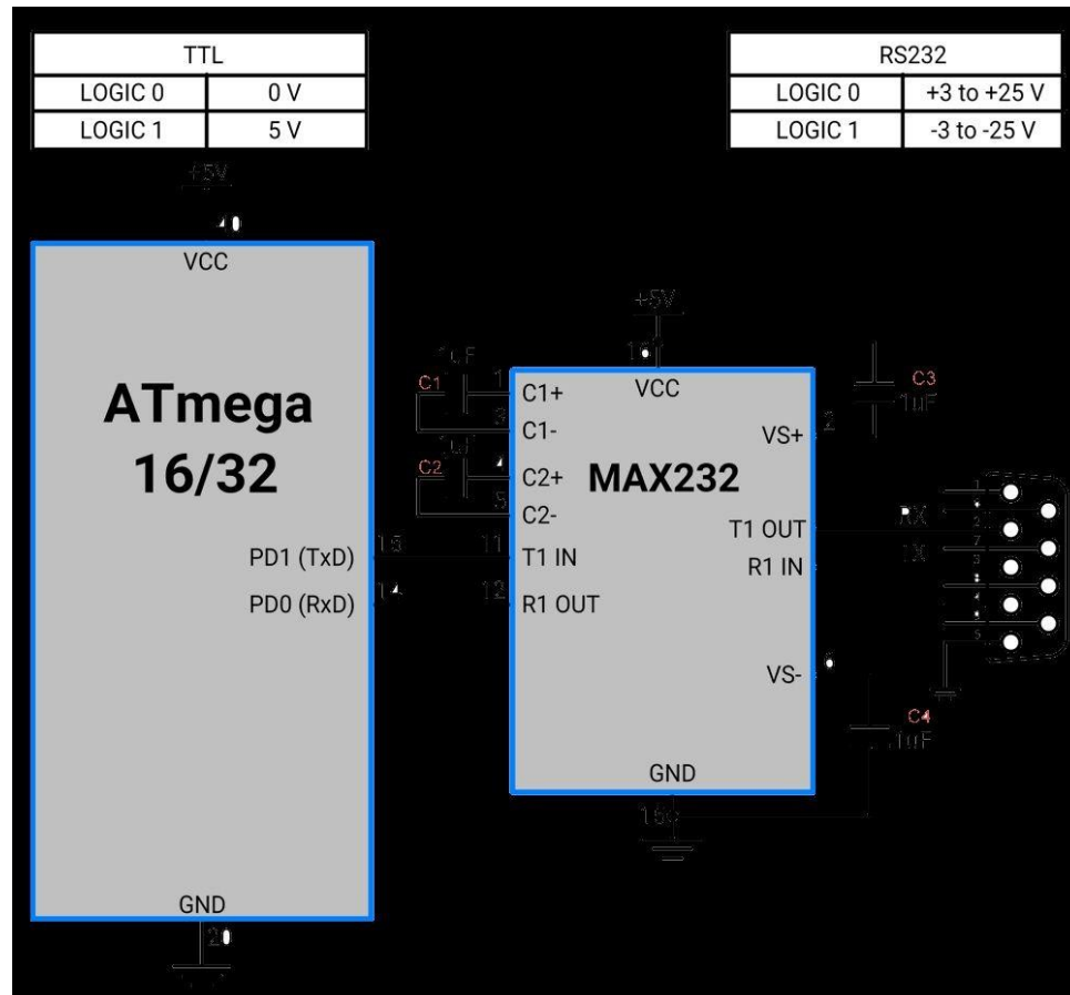
ATmega16/32 Serial Interface Connection Diagram
